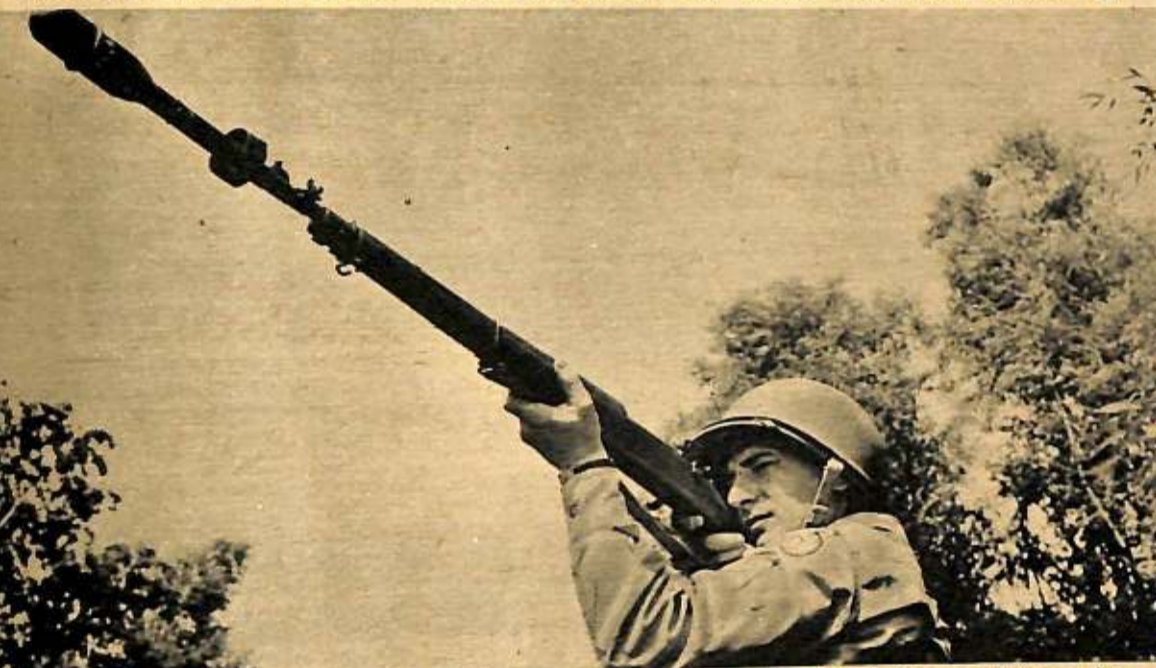
RIFLE GRENADE. Add a launcher-adaptor to an Army 30-caliber and it can be quickly turned into a high-powered grenade thrower. A rifle so equipped can reach the areas not covered by hand grenades and is especially effective against pillboxes.
