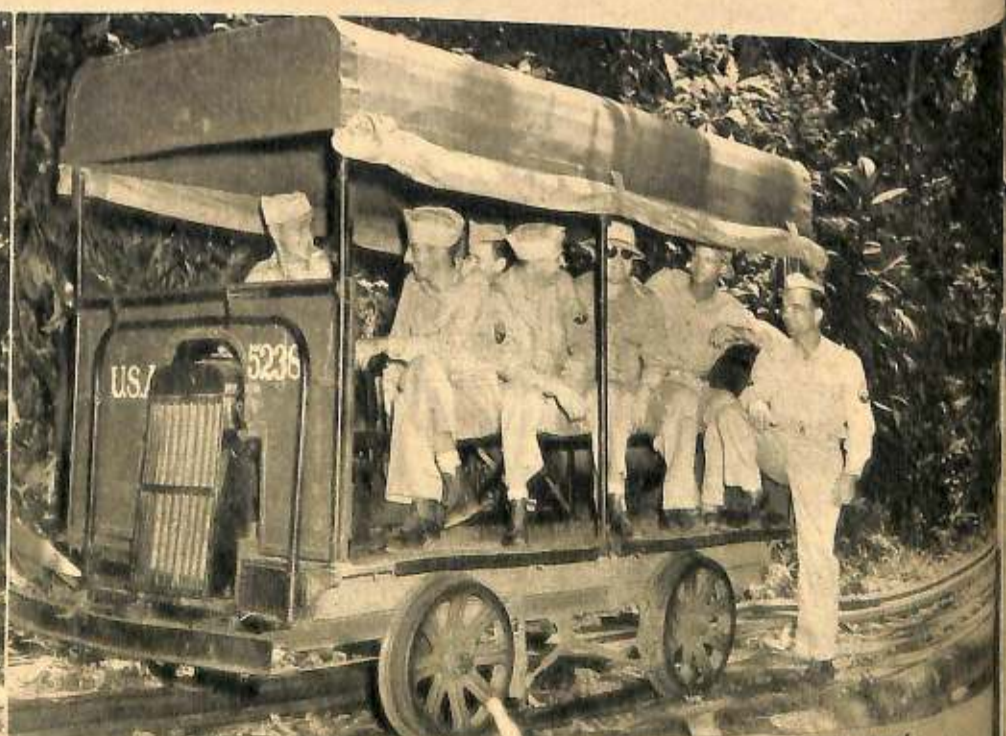
This GI skooter, made from a flat car and a V-8 engine, carries Yanks back and forth from jungle outposts and base camps. Here the skooter, a bouncing vehicle of uncertain moods, has picked up some passengers at a jungle stop.
