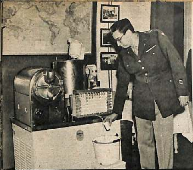
ROBOT COW. LT. COL. JAMES R. KARR SAMPLES SOME MILK MADE OUT OF POWDER, WATER AND BUTTER BY THIS MECHANICAL GADGET, WHICH CAN MAKE ICE CREAM, TOO.
