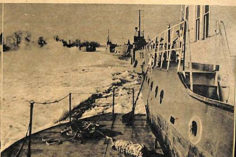
WEATHER. Grumblers in the ETO, take note: This U. S. Coast Guard ice breaker is smashing the ice of the frozen upper Mississippi to free newly built LCT vessels scheduled to leave for combat zones.
