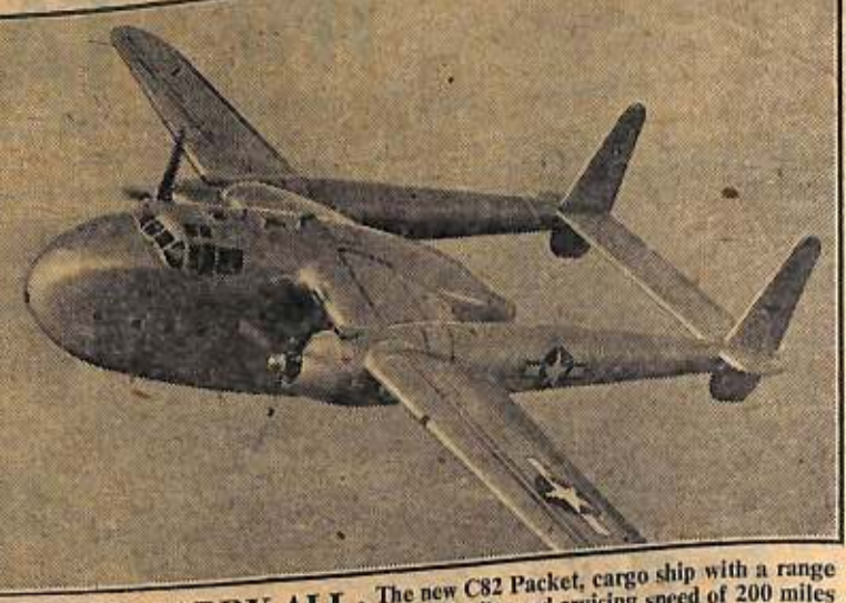
WINGED CARRY-ALL: The new C82 Packet, cargo ship with a range of 4,000 miles and cruising speed of 200 miles per hour, can carry trucks, tanks, jeeps, light artillery and other military supplies.
